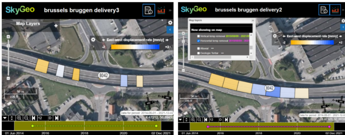
Figure 11. Decomposition of S1 ascending and descending into horizontal displacements on bridge segments (westward movements in orange and eastwards movements in blue). Left: area in between the pillars with a 5 m buffer on either side. Right: bridge segments with no buffer around the pillars.
