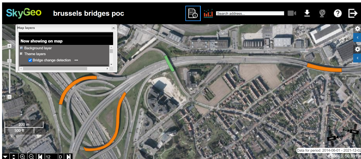
Figure 10. Alerting system in SkyGeo Maps, in the same viewer. For the PoC bridges are coloured based on amplitude (yellow), change in displacement rate (orange), a change in amplitude and displacement rate (red) or no change at all (green). This view can also be integrated into the catalog for end-users with access rights to see the report per bridge and or the underlying InSAR data.
